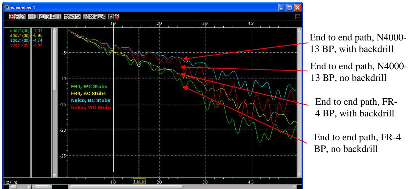
Figure 2 Insertion loss of end-to-end path – 4” modules and 12” backplane
